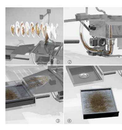
**Phase**  $\odot$ : Coarse soiling is removed from the wash ware early, in the pre-wash zone.
